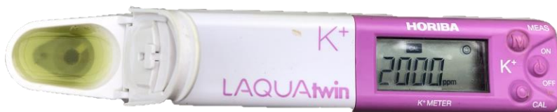
Figure 3. (Below) Showing petiole sap on the sensor and the reading achieved.
